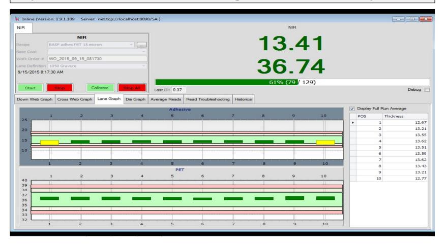
In-process measurement of base film and applied wet adhesive layer
