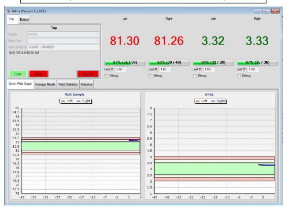
Multiple recipes can be defined for different probe sets, top and bottom
