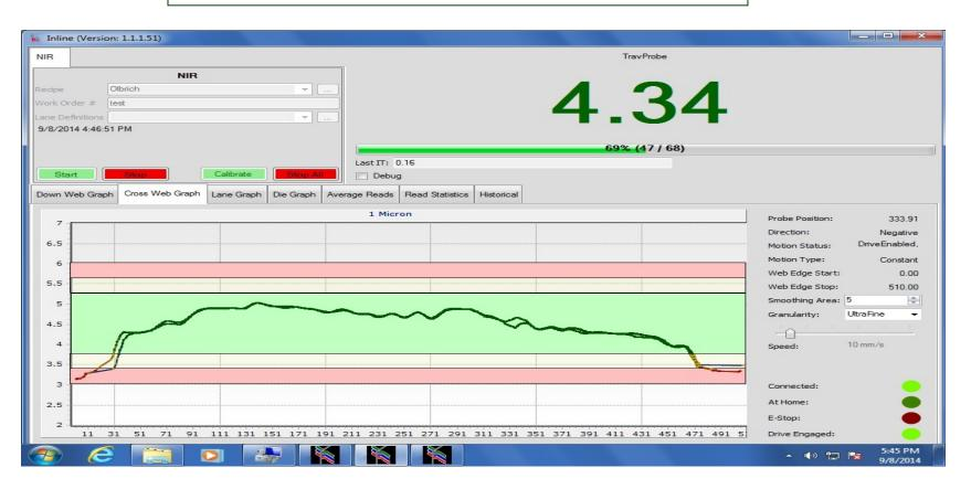
Weight checks can miss web variations that can be detected with in-line tools
