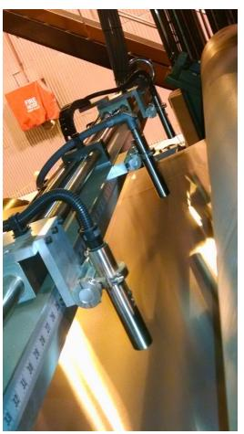
Regularly used for in-process coating measurement on metal and webs
