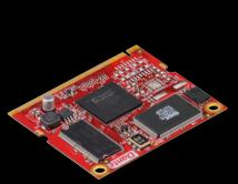
Audinate's Brooklyn provides all the core networking, control and monitoring functions needed for products such as DSP processors, amplifiers, digital snakes and break-in/break-out boxes, allowing manufacturers to more easily develop Dante-enabled products.
